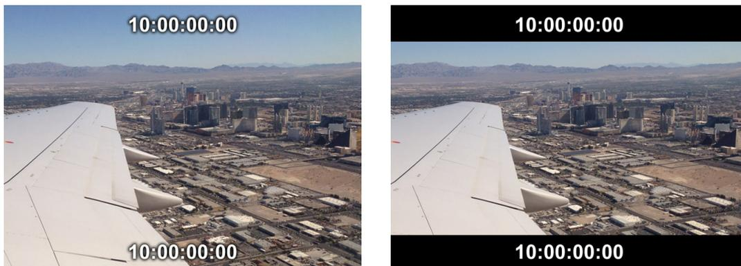
Figure 5-20: Burnt-in timecode in the record file
