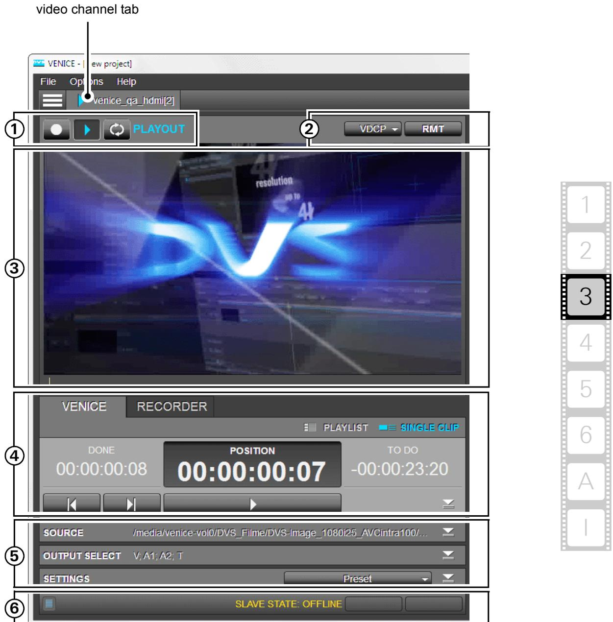
Figure 3-9: The video channel tab in playout mode
